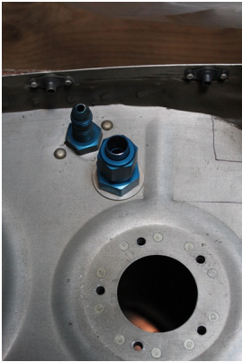
Return line (lower) using Earls Stat-o-seals
