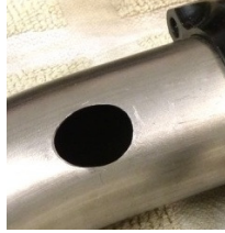
Make oval hole in induction tube
