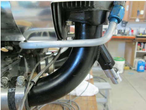
Injector boss welded in place ( Lycoming)
