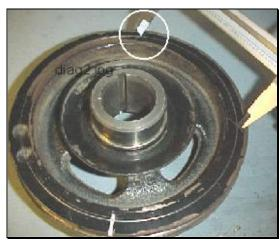
Scribe another arc at the top. This point is 180 degrees from the #1 mark on the pulley. This point can be center punched for drilling.
