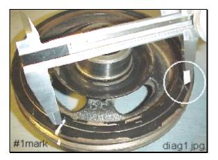
Scribe another arc at the top. This point is 180 degrees from the #1Trigger magnet mark on the pulley. This point can be center punched for drilling.
