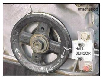
In this example, the engine rotates clockwise as shown by the arrow marked on the pulley. If this engine happened to rotate counter-clockwise, like a front-drive Honda, then the #1 magnet mark would be at roughly the one-o'clock position on this particular engine shown.
