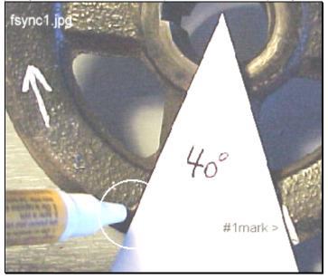
Using a marking pen, draw the sync magnet mark through the belt groove around to the back side of the pulley. In this installation the magnet will be in the back side.
