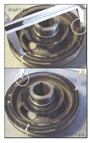
Scribe an arc with calipers and center punch this location for drilling.
