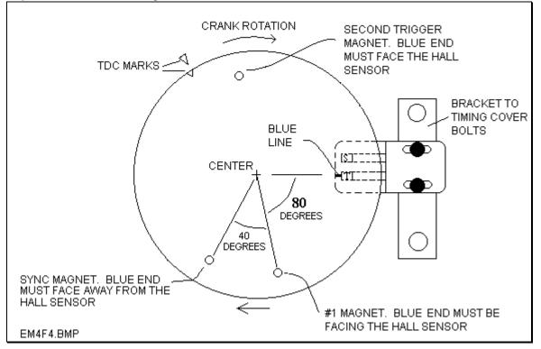
6 cylinder schematic drawing of hall sensor installation.
