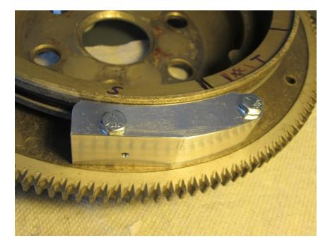
7. Now, move drilling block over so that drilling hole is close to the "TC #1" mark on rear of flywheel. The block should be over holes 12 and 1. See photo below.
