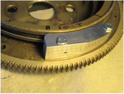
4. Verify that the center of the drill bit is in the center of the flywheel shoulder before you start drilling. You can rotate the bit by hand and see where the mark is. If correct, tighten the nuts so that the block is held firmly in place before drilling.
