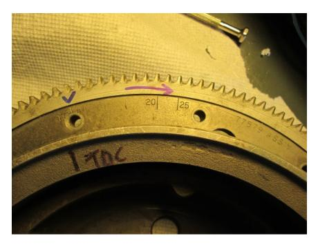
2. Now viewing the flywheel from the back side, counting the hole closest to the TC#1 mark as 1, use marker to mark all twelve ¼ inch flywheel holes as shown below:
