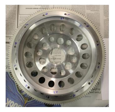
3. Count over 6 holes in the direction of crankshaft rotation (clockwise as viewed from the BACK of the flywheel). Line the round edge of the drilling block with this hole, slip the supplied bolts through the block and holes 6 and 7 as shown below.
