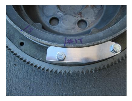
3. Use the supplied #29 drill to drill through the drilling block and flywheel as shown below. Lubricate the drill and remove frequently to clean out the chips. Mark the flywheel close to the hole as "#1T" with marker.
