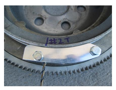
6. This is the #2 Trigger Magnet hole and should be 120 degrees across from the #1 Trigger Magnet hole. Mark this hole as "#2T". Drill through the flywheel.
