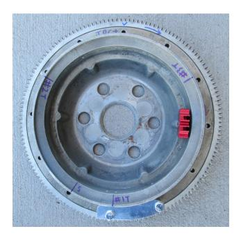
We recommend that you number each of the twelve ¼ inch holes in the flywheel with marker as shown below starting at the TC#1 hole as 1.
