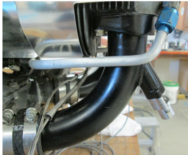
Injector boss welded in place ( Lycoming)
