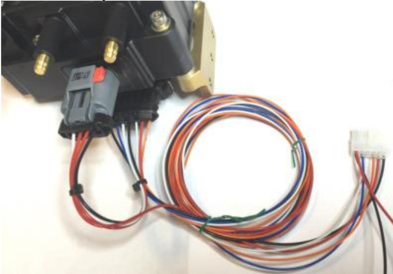
Insert red, black, orange, white and blue (6cyl) terminals into 12pos white plug after you've routed and passed these through the firewall.
