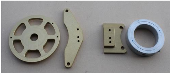
Rotax magnet disc and Hall mount left, Jabiru right
