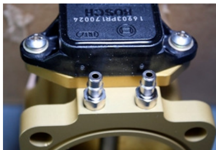
Throttle body fittings on 60 and 80mm models for connecting fuel pressure regulator and MAP sensor
