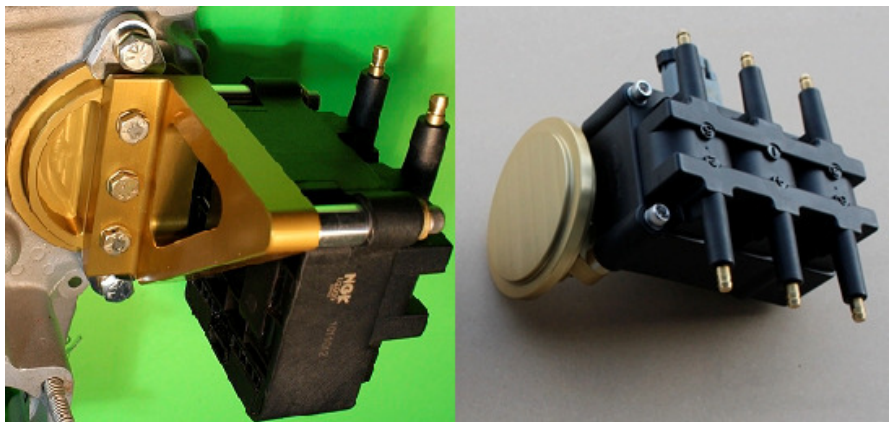
4 cylinder and 6 cylinder coilpacks with rear mag mounts
