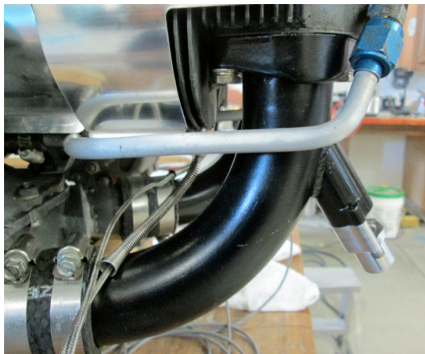
Injector boss welded in place (Lycoming)
