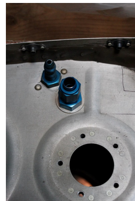
Return line using Earls Stat-o-seals
