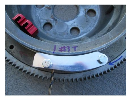
Remove the drilling block and insert the supplied 8-32 tap, lubricated with tap oil, into each drilled hole. CAREFULLY tap until the tip of the tap is flush with the ID of the flywheel, don't tap all the way through. Break the chips on every turn of the tap and clean the tap and hole of chips with compressed air frequently to prevent jamming and breaking the tap. Clean the holes out with acetone to remove all traces of oil.
