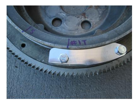
3. Use the supplied #29 drill to drill through the drilling block and flywheel as shown below. Lubricate the drill and remove frequently to clean out the chips. Mark the flywheel close to the hole as "#1T" with marker.
