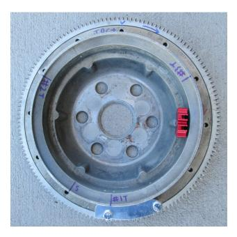
We recommend that you number each of the twelve <sup>1</sup>/<sub>4</sub> inch holes in the flywheel with marker as shown below starting at the TC#1 hole as 1.
