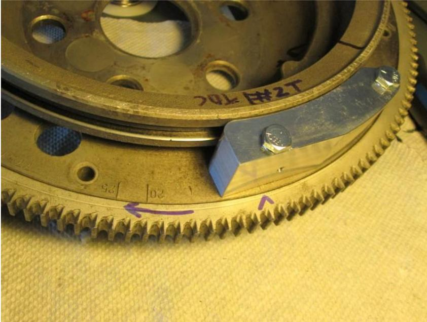
6. This is the #2 Trigger Magnet hole and should be 180 degrees across from the #1 Trigger Magnet hole. Mark this hole as “2T”. Drill through the flywheel.
