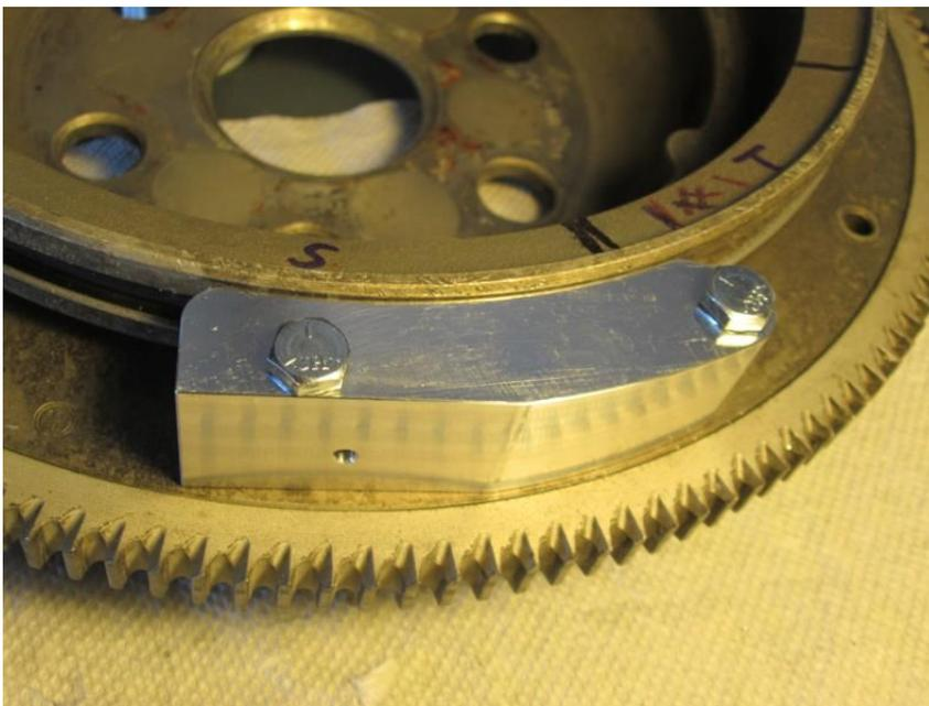
5. Now, move drilling block over so that drilling hole is close to the “TC #1” mark on rear of flywheel. See photo below.
