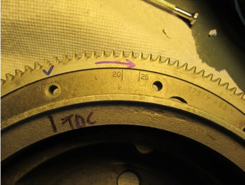
2. Now viewing the flywheel from the back side, counting the hole closest to the TC#1 mark as 1, count over 6 holes in the direction of crankshaft rotation (clockwise as viewed from the BACK of the flywheel). Line the round edge of the drilling block with this hole, slip the supplied bolts through the block and holes 6 and 7 as shown below.
